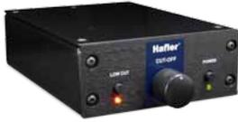
Integrated amplifiers are a combination of the preamp stage (including input switching) and the power amplifier stage in a single unit. This component is most common as it requires less space but does not allow the listener to tailor the sound to the same degree.
