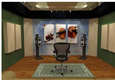
The optimal listening position is one corner of an equilateral triangle created along with the 2 speakers. In 2.1 systems the placement of the sub-woofer is not a critical. Low frequencies are omnidirectional and as frequencies go higher, the sound is more directional. For example if your speaker are 8ft apart you should be 8ft from the center of the speakers
